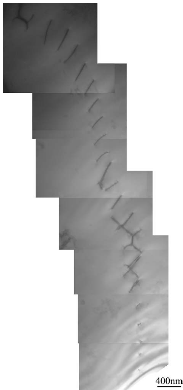
Figure 7 Bright field TEM image of a periodic array of dislocations forming a low angle GB.
